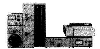
• Jasco Inc. has introduced the Tri Rotar, a pumping system permitting use of the single instrument for gradient work, resulting in increased baseline stability and detection, the firm says. Typical pump outputs range from 0.1 ml/min to 9.9 ml/min in 0.1 min steps with a flow accuracy of 1 percent. Operation is at 7100 psig (500 KG/cm<sup>2</sup>). Information: J. Bambling, Jasco Inc., 218 Bay St., Easton, MD 21601 (tele: 301-822-1220).
