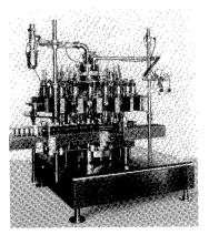
• Horix Manufacturing Co. has introduced Var-I-Vol, a positive displacement liquid filler. The Var-I-Vol features a volume adjustment rod that provides first-step volume adjustment to within 5 percent of required fill volume, the firm says, followed by fine-tuning adjustment of the precision volume adjustment knob for precise volume delivery of each individual chamber. Information: Horix Manufacturing Co., Pittsburgh, PA 15225.
